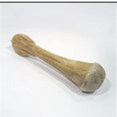
EPS Peanuts + Acrylic Sphere + Acetone Casting + Hanging
