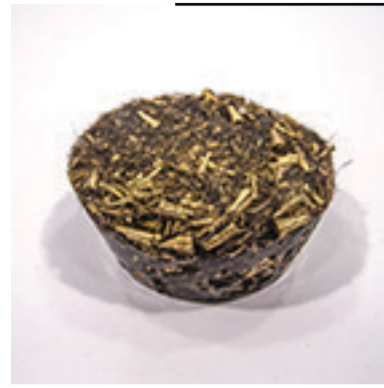
Chopped Hair + Brass Shavings + Epoxy Mixing + Casting
