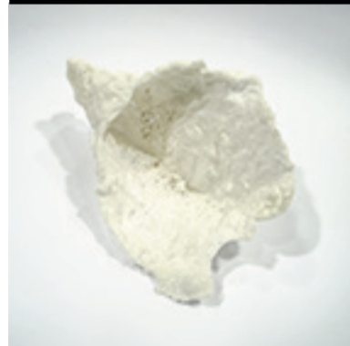
EPS + Acetone Shaped + Heat Puffed
