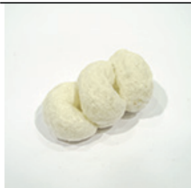
EPS + Acetone Shaped + Heat Puffed
