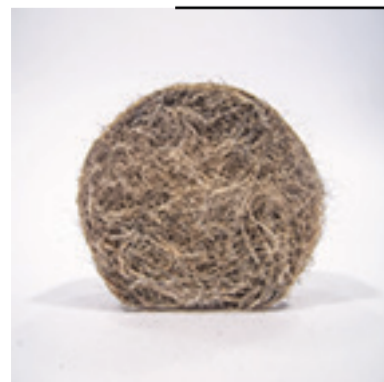
Hair + Epoxy Mixing + Casting
