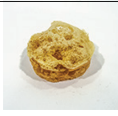
PU Foam + Acetone Dissolving + Boiling
