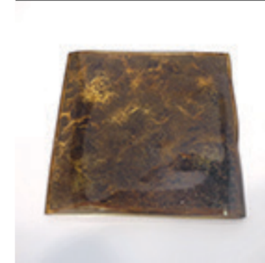
Thick Plastic Sheet Burning to Texturize
