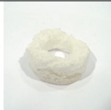
EPS + Acetone + Ink Brushed on Silicon Mat + Heat Puffed + Sanded
