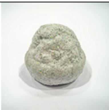
EPS + Acetone + Glitter Heat Puffed from 2 Sides
