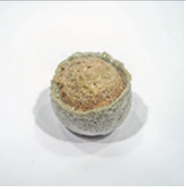
EPS + Acetone + Glitter Heat Puffed + Scooping + Casting + Heat Puffed
