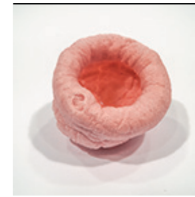
EPS + Acetone Shaped + Heat Puffed
