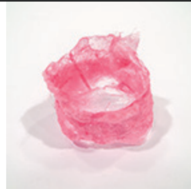
EPS + Acetone + Ink Brushed on Silicon Mat + Heat Dried
