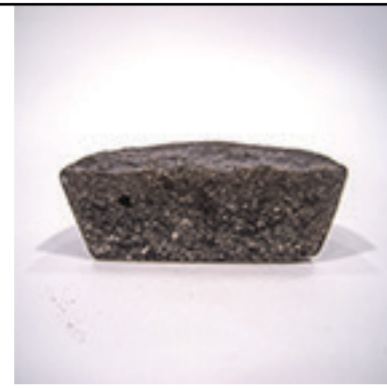
Chopped Hair + Epoxy Casting + Cutting + Polishing
