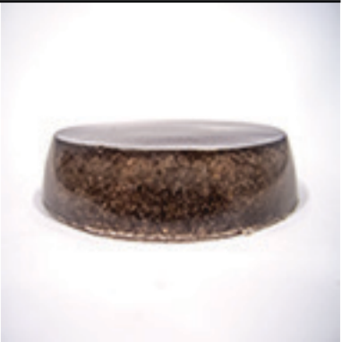
Chopped Hair + Epoxy Casting by Layering
