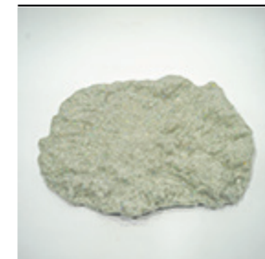
EPS + Acetone + Glitter Mixing + Dissolving + Heat Puffed
