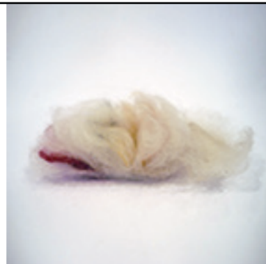
Wool + Medium Plastic Sheet Punching
