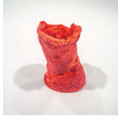
EPS + Acetone + Ink Shaped + Heat Puffed Inside Only
