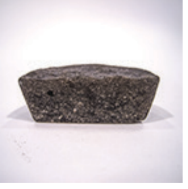
Chopped Hair + Epoxy Casting + Cutting + Polishing
