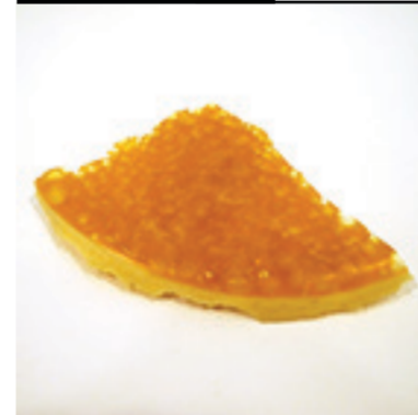
PU Foam + Acetone Casted + Left to Dry
