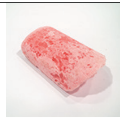
EPS + Acetone + Ink Heat Puffed + Sanded
