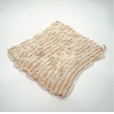
EPS + Acetone + Copper Thread Dissolving + Smearing Heat Puffed + Knitting
