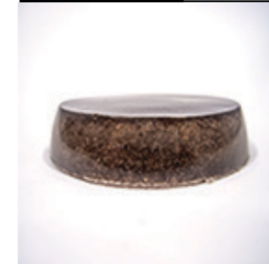
Hair + Epoxy Casting by Layering
