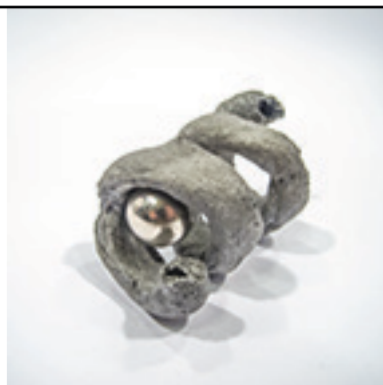
EPS + Acetone + Metal Dust Molded Around Metal + Heat Puffed
