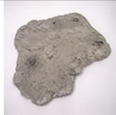
EPS + Acetone + Metal Dust Spread + Left to Dry
