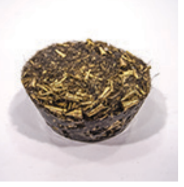
Chopped Hair + Brass Shavings + Epoxy Mixing + Casting
