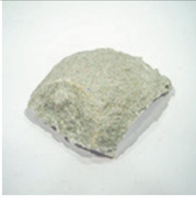
EPS + Acetone + Glitter Coated on Ceramics + Heat Puffed
