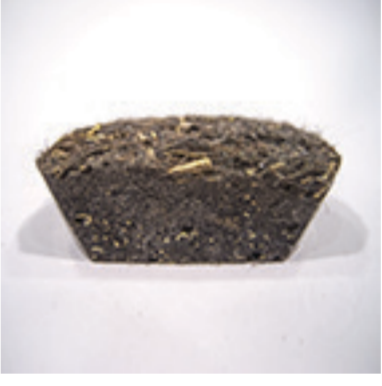
Chopped Hair + Brass Shavings + Epoxy Casting + Cut + Polishing
