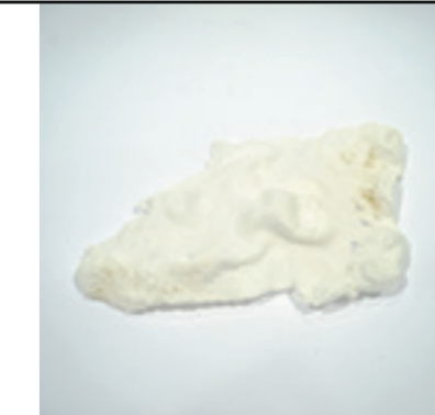
EPS + Acetone Dissolving + Dried + Heat Gun
