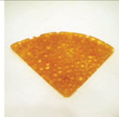
PU Foam + Acetone Casting + Dried + Sanded
