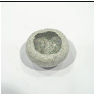
EPS + Acetone + Glitter Heat Puffed + Scooping
