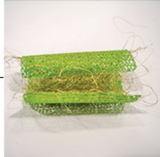
Styrofoam + Acetone Dissolving + Casting
