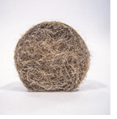
Hair + Epoxy Mixing + Casting
